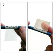
Wrap the clear area around the wire, covering the printed area.
